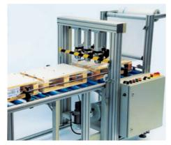
Nailing station with stapling heads C 13-30/80. Foils or carton are nailed fully automatically onto wooden pallets. The feed travel up to 80 mm compensates different pallet heights.
