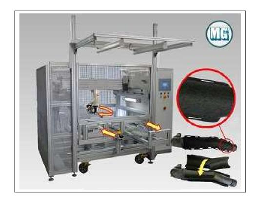
Clinching tables are mounted in two pull-out drawers. The first component (pipe/acoustic cap) will be inserted into drawer 1 and fixed by a lever. The complete sliding component will be inserted into the stapling area. By means of the START push-button the clinching process will be released. The sliding axle drives the stapling head into the programmed positions to achieve the fastening of the plastic cap.
