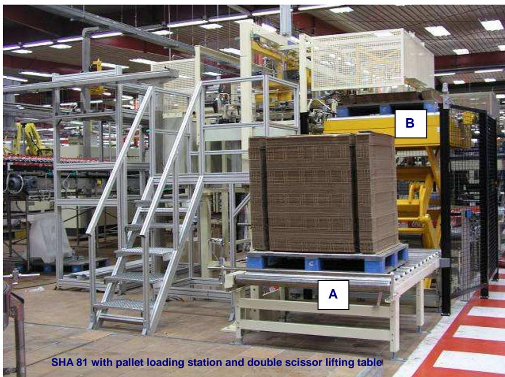
SHA 81 with pallet loading station and double scissor lifting table
